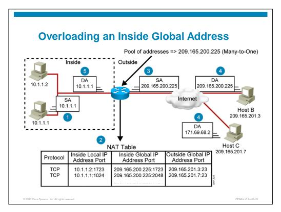
As described earlier, PAT or NAT overload deploys the same five-step process as before, except that the source and destination UPD/TCP port number is recorded along with the IP address as part of the translation. This is how thousands of inside local IP hosts may be translated to one inside global host.
