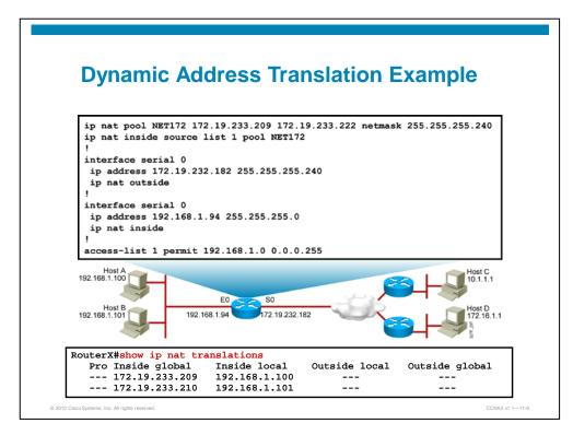
The graphic shows a completed dynamic NAT configuration. Note that the translation configuration line includes a network mask or prefix following the address pool.
