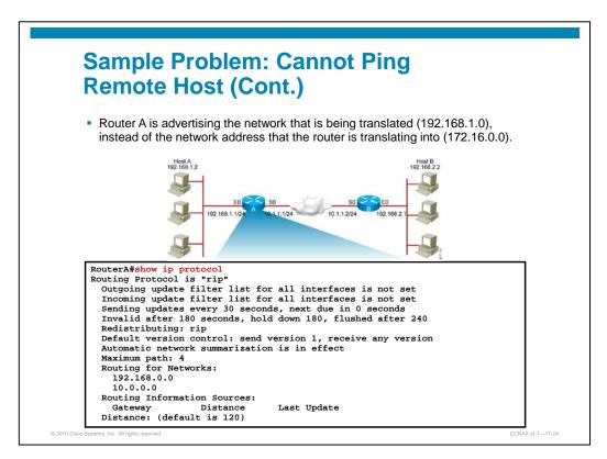
On Router A, the **show ip protocols** command verifies that there is no network statement for 172.16.0.0 configured. The graphic shows the corrected configuration.
