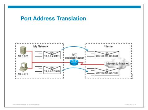
The graphic further clarifies the idea of PAT. Along with the inside local address to be translated to an inside global address as the packet exits the router, the port number (both source and destination) is recorded. In the case where non-TCP packets are used, such as ping packets, NAT/PAT creates a source and destination port. This enables several thousand inside local hosts to be translated to one inside global host IP address.
