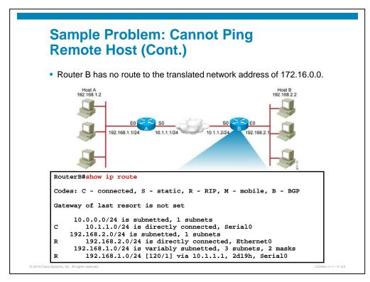
A check of the routing table on router B verifies that there is no route back to the 172.16.0.0 network.
