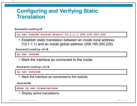
The graphic illustrates the commands used to configure static NAT:
