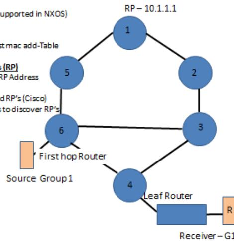
1. Receiver sends an IGMP join to its leaf router to join Group 1
